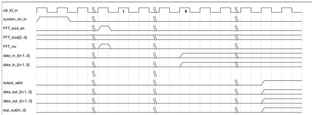
At any time after system\_rst\_in goes low, FFT\_en is used to latch the direction of the transform (FFT\_inv=0/1 for forward/inverse). Following this, the circuit expects to see continuous data appearing on the 8th subsequent cycle. Valid data out occurs when output\_valid (output\_en) goes high. For streaming operation output is continuous from this point on.
