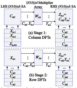
Fig. 2. Systolic processing flow for column and row DFTs. Subscript "c" and "r" refer to computing column and row DFTs of the  $N_3 x N_4$  DFT matrix.
