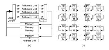
Fig. 1(a). Traditional memory-based FFT architecture and (b) fine-grained SA equivalent.
