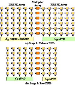
Fig. 5. Virtual 2-D arrays used for row and column DFTs, *N*=520. TABLE IV. DFT PERFORMANCE BASED ON CYCLE COUNTS.
